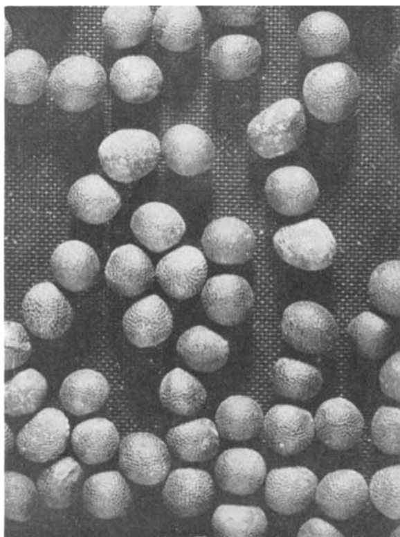
Fig. 2. Mustard seeds, 1,545\mu , on 200-mesh screen.
